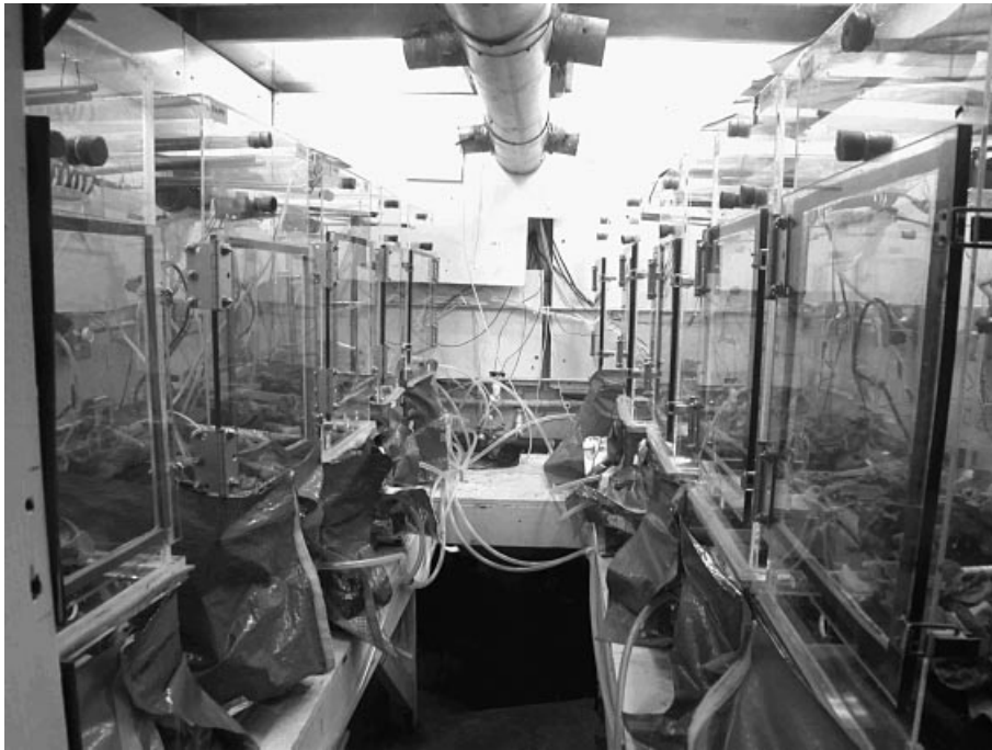
FIG. 1. The ten-chamber gas-exchange system. There are five chambers on each side of a walk-in growth chamber. Each chamber has a reflective skirt wrapped around the outside to minimize side lighting.
